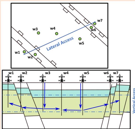
Sample parameters collected to determine **Zone of impact**: lateral and vertical reservoir access:
